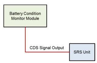
Collision Power Shutdown System Diagram
