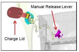
Accord Plug-In Charge Lid & Manual Release Lever
